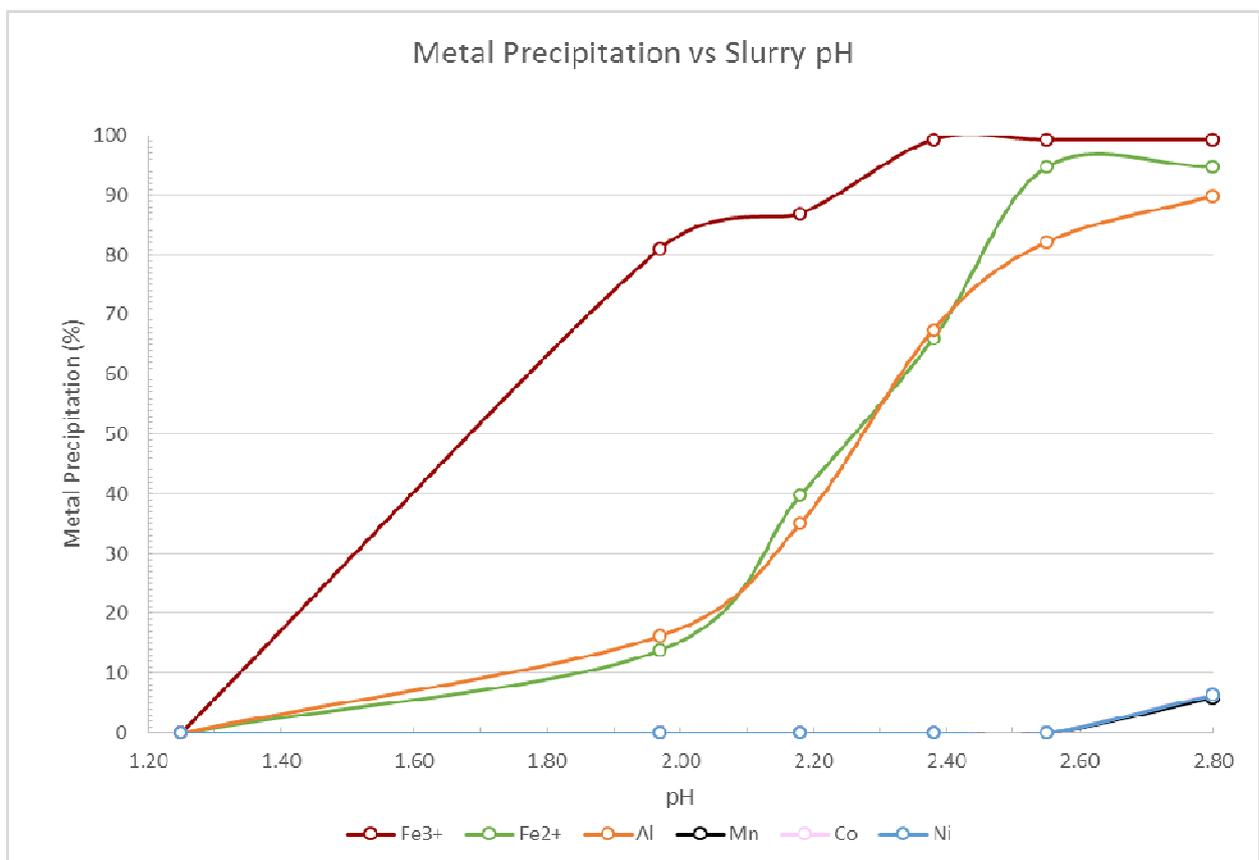
**Figure 3: Neutralisation test HY7252 showing successful precipitation of iron an aluminium ahead of payable metal precipitation at pH 2.4-2.6.**
