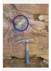
Above: Example of a massive sulphide globule at surface believed to have been locally remobilised from a massive sulphide body nearby
